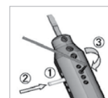
Fig. 1: How to Use Adjustment Pin
