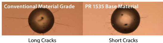
Cracking Comparison by Diamond Indenter (Internal Evaluation)
